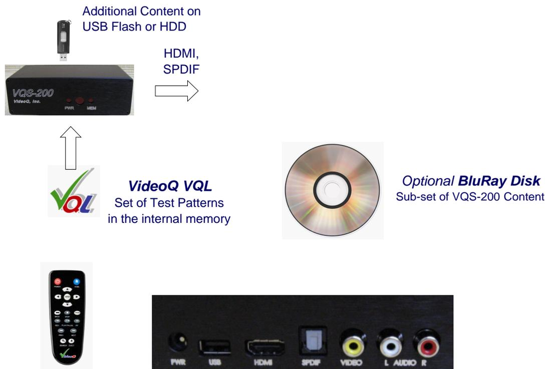
VQS-200 is equipped with digital HDMI and SPDIF outputs plus baseband analog NTSC/PAL CVBS video output and analog L-R audio outputs.
